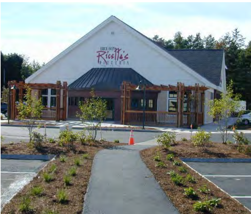
An internal walkway oriented toward the main entry of a restaurant in a multiple building development. The planting strips with ornamental grasses and perennials separate the pathway from overhanging bumpers.
