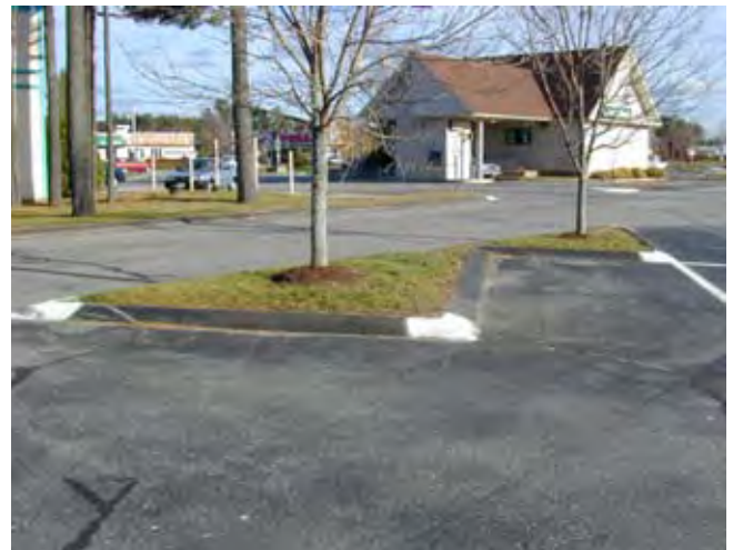
Trees can be planted throughout parking lots as long as they are given enough room for proper root development and protection from cars and snowplows.
