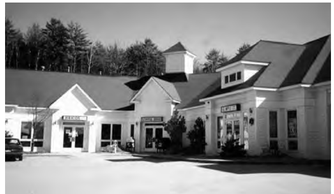
The scale of this commercial building has been effectively reduced through variations in its roofline and projecting gables.
