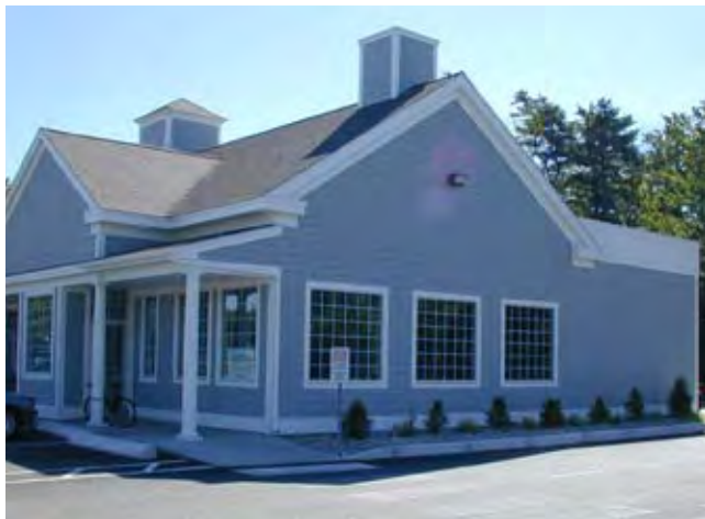
The facade treatment on this shop wraps around the corner to present a unified design from all visible faces. The entrance is emphasized by columns and the lower roofline.
