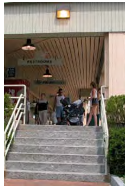
Unshielded wall-pack lighting can cause dangerous glare and make it difficult to see the stairway.
