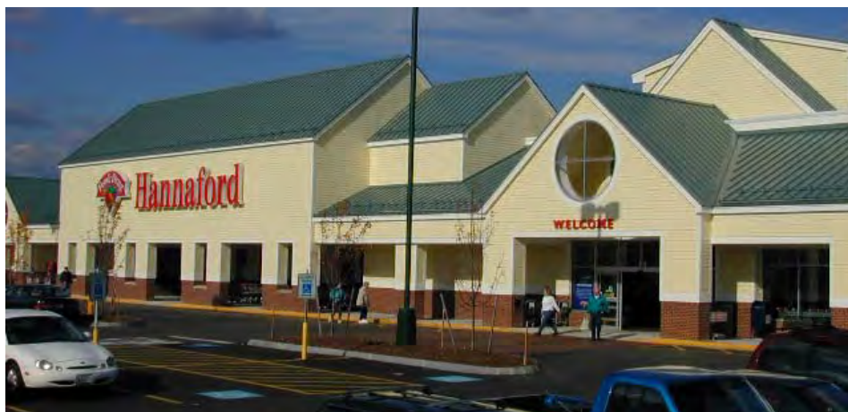
Large retail buildings can be designed to avoid the appearance of a ‘big box’ through careful massing and detailing.
