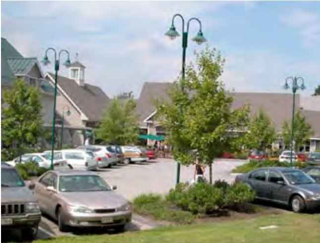
A well-coordinated lighting plan that uses variations on the same fixture for both walkway and parking lot lighting.
