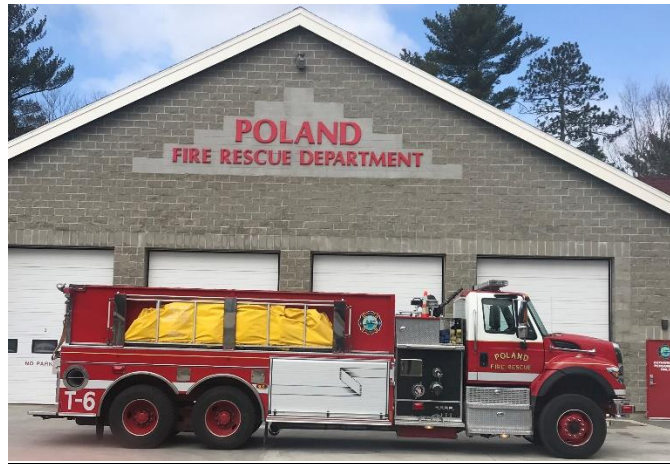
Tank-6 which is a 2009 International/Pierce 2500 gallon tanker.
