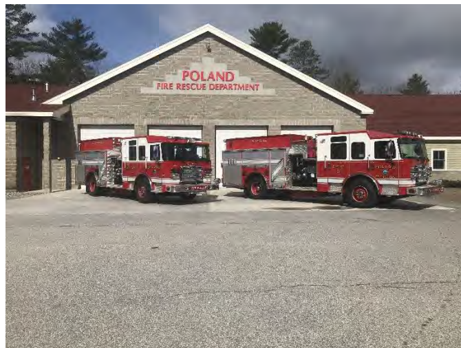
Our fleet of Engines, Engine 2(2016) and Engine 3 (2015) Pierce Enforcers. Each with 1500 GPM pumps, 1000 gallons of water on board. (Above Photo)
