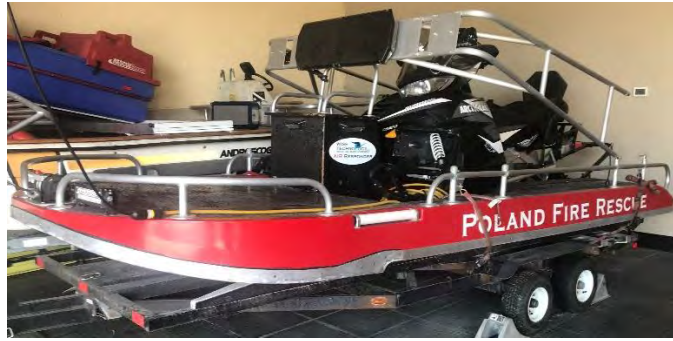
Air Responder, combination ice/water rescue vehicle with an Arctic Cat snowmobile (Above Photo)
