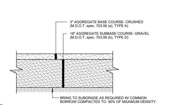
1. COMPACT GRAVEL SUBBASE COURSE TO 92% OF MAXIMUM DENSITY USING HEAVY ROLLER COMPACTION. 2. CONTRACTOR SHALL SET GRADE STAKES MARKING SUBBASE AND FINISH GRADE
