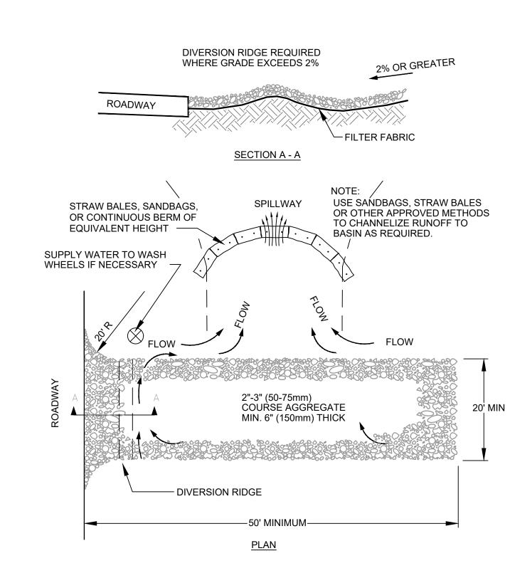
1. THE ENTRANCE SHALL BE MAINTAINED IN A CONDITION THAT WILL PREVENT TRACKING OR FLOWING OF SEDIMENT ONTO PUBLIC RIGHT-OF-WAYS. THIS MAY REQUIRE TOP DRESSING, REPAIR AND/OR CLEAN OUT OF ANY MEASURES USED TO TRAP SEDIMENT.
