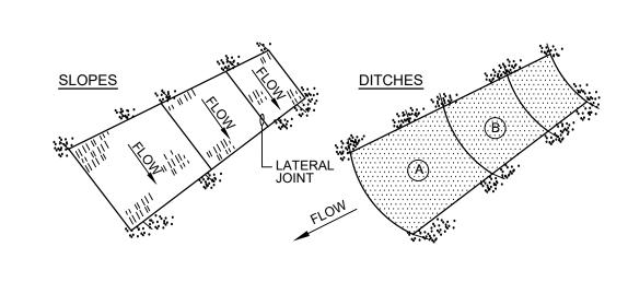
WITH STAPLES AT 6" SPACING, 4" DOWN FROM EXPOSED END.
