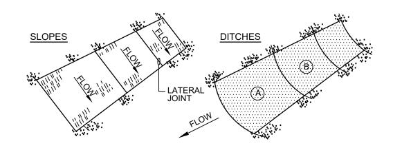
1. BURY THE TOP END OF THE MESH MATERIAL IN A 6" TRENCH AND BACKFILL AND TAMP TRENCHING SECURE END WITH STAPLES AT 6" SPACING, 4" DOWN FROM EXPOSED END.
