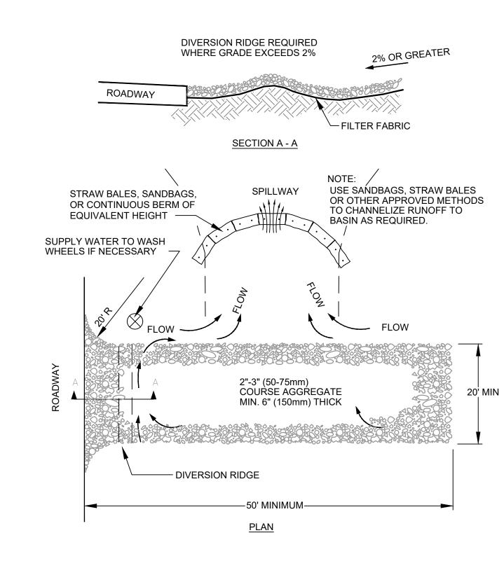
1. THE ENTRANCE SHALL BE MAINTAINED IN A CONDITION THAT WILL PREVENT TRACKING OR FLOWING OF SEDIMENT ONTO PUBLIC RIGHT-OF-WAYS. THIS MAY REQUIRE TOP DRESSING, REPAIR AND/OR CLEAN OUT OF ANY MEASURES USED TO TRAP SEDIMENT.
