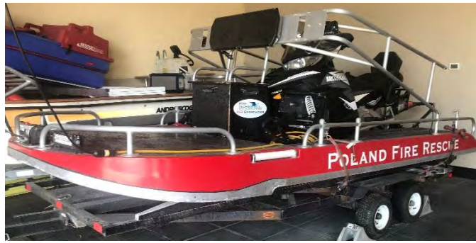
Air Responder, combination ice/water rescue vehicle with an Arctic Cat snowmobile
